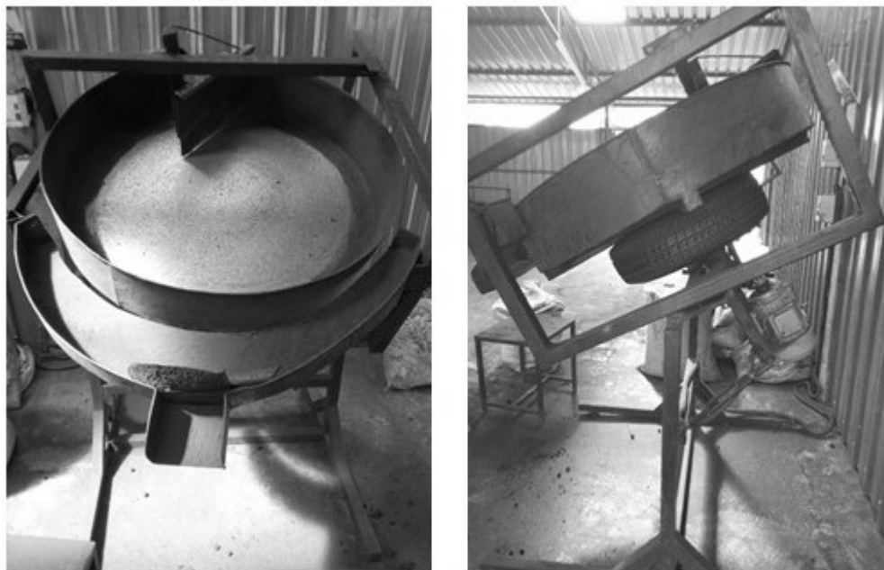
Figure 2: Rotating briquette maker from NAWASSCO (Source: NAWASSCO with permission).
