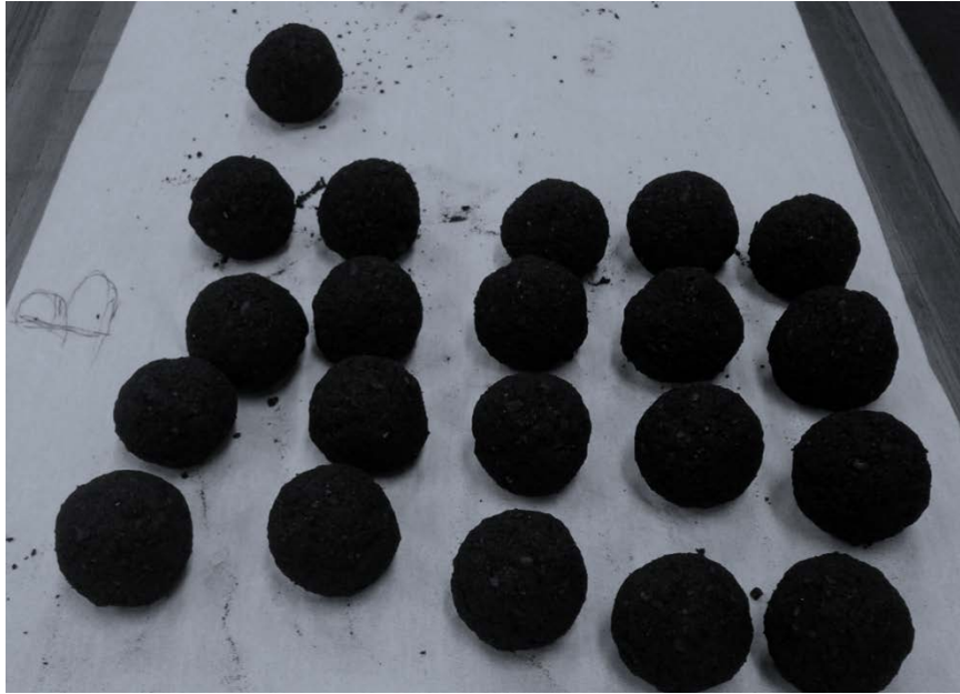
Figure 5: Hand molded briquettes made in the laboratory at TUT.
